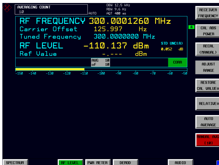
Fig.2-8 Tuned RF Level measurement with Averaging
